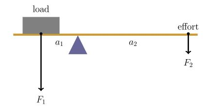
The lever is in balance when the torque of the load equals to that of the effort.
