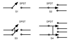
All homes have separate *hot/live* and *neutral* busbars in the circuit-breaker that connect to all the electronics in your home. When a path exists between hot and neutral, current flows freely and any devices along that path turn on. Switches work by manipulating those paths. Below is an example of a simple circuit with a SPST switch that turns a lightbulb on and off.
