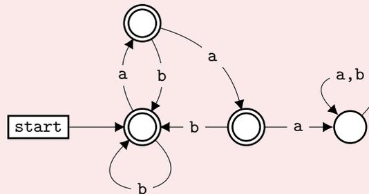
This automaton rejects all strings with three 'a's in a row. If we count accepted strings, we get the Tribonacci numbers with an offset:  $f(0) = 1, f(1) = 2, f(2) = 4, \dots$
