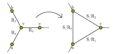
Show that if  $S = R_1R_2 + R_1R_3 + R_2R_3$ , the effective resistance between any two of a, b, c are the same for both circuits. (It is often useful to turn one of these circuits into the other!)
