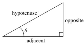
The right angle is denoted by the square, while another angle is labelled  $\theta$ . The adjacent side is the "straight" edge that sits next to  $\angle\theta$ , while the opposite side is the edge that  $\angle\theta$  opens into. The hypotenuse is the longest side.
